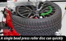
A single bead press roller disc can quickly assist mounting and demounting stiff sidewall tires.
