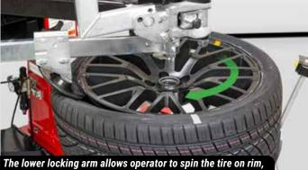
The lower locking arm allows operator to spin the tire on rim, helping match-mount low spot on rim to stiffest point on tire.
