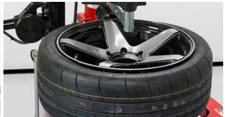
Upper roller can lock or freewheel, offering assistance in every situation.
