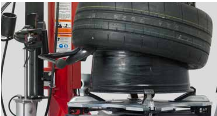
Demount heavy, stiff, or wide tires easily with locking lower disc.
