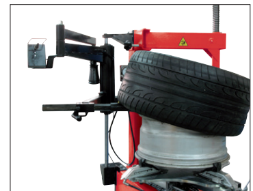
Helper arm demounting lower bead
