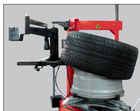
SHOWN: Helper arm demounting lower bead
